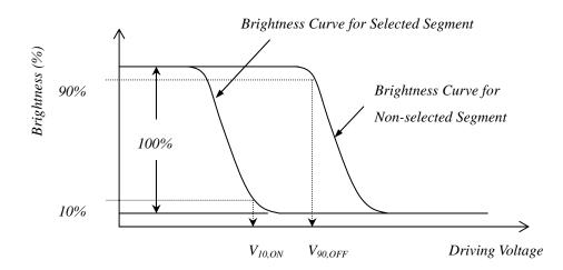
$Vop = (V_{10,ON} + V_{90,OFF})/2$
