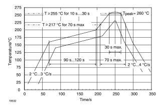
Figure 5. Solder Profile, RSS Recommendation
