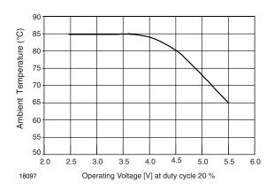
Figure 3. Current Derating Diagram
