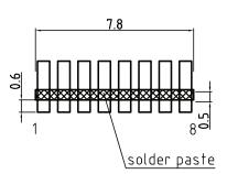
Figure 9. Recommended footprint for top view applications and solderpaste mask
