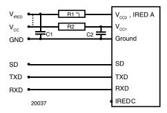
Figure 1. Recommended test circuit.
