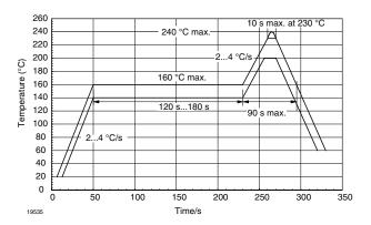
Figure 4. Recommended Solder Profile for Sn/Pb soldering
