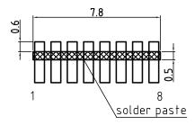
Figure 8. Recommended footprint for side view applications and solderpaste mask
