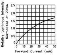
Fig.4 RELATIVE LUMINOUS INTENSITY VS. FORWARD CURRENT
