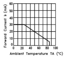
Fig.3 FORWARD CURRENT DERATING CURVE
