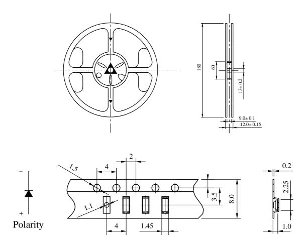
Reel Lead Min.60mm No LEDs
