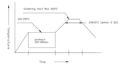
3. Reflow SolderingPreheating:140Operation heating:235Gradual Cooling (Avoid quenching)
