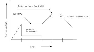
3. Reflow SolderingPreheating:140Operation heating:235Gradual Cooling (Avoid quenching)
