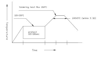
3. Reflow SolderingPreheating:140Operation heating:235Gradual Cooling (Avoid quenching)
