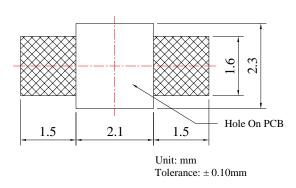
1. Soldering terminal may shift in x, y direction.
