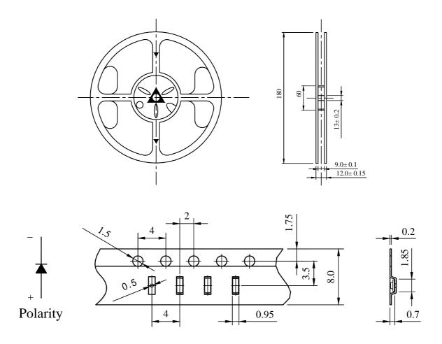
Reel Lead Min.60mm No LEDs
