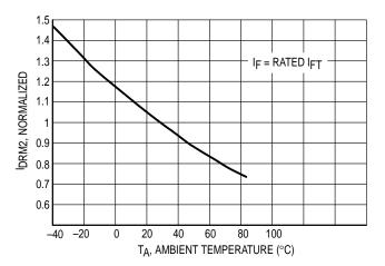
Figure 4. I<sub>DRM2</sub>, Leakage in Inhibit State versus Temperature
