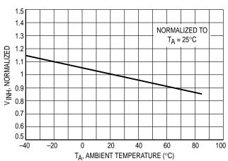
Figure 2. Inhibit Voltage versus Temperature
