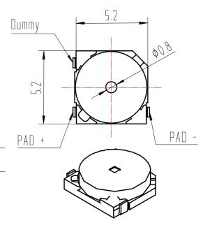
\*Unit: mm; Tolerance: ± 0.3mm Except Specified \*Housing Material: Black LCP Top(Brass) \*Terminal plate: 3 soldering pads, tin Plating Brass
