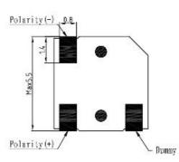
\*Unit: mm; Tolerance: ±0.3mm Except Specified
