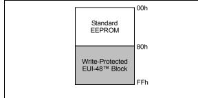
The 6-byte EUI-48 node address value is stored in array locations 0xFA through 0xFF, as shown in Figure 9-2. The first 3 bytes are the Organizationally Unique Identifier (OUI) assigned to Microchip by the IEEE Registration Authority. Microchip's OUI is 0x0004A3. The remaining 3 bytes are the Extension Identifier, and are generated by Microchip to ensure a globally-unique, 48-bit value.
