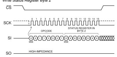
Figure 11-3. Write Status Register Byte 2
