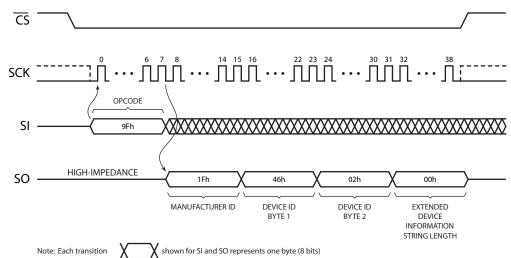
Figure 12-2. Read Manufacturer and Device ID
