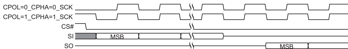
Figure 3.1 SPI Modes Supported
