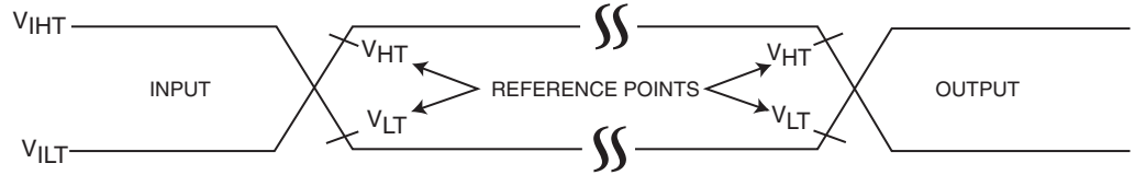
FIGURE 8-5: AC INPUT/OUTPUT REFERENCE WAVEFORMS
