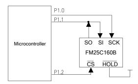
Figure 3. System Configuration without SPI port
