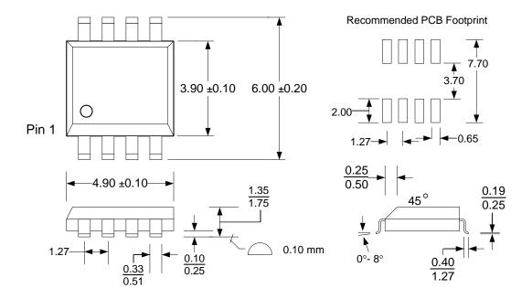
Refer to JEDEC MS-012 for complete dimensions and notes. All dimensions in <u>millimeters</u>.
