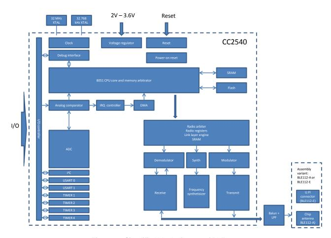
Figure 17: Simplified block diagram of BLE113
