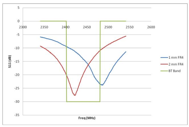
Figure 15: Typical return loss of BLE113-A with two different mother board PCB thickness
