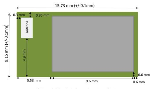
Figure 8: Physical dimensions (top view)
