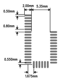
Figure 10: Recommended land pattern for BLE113-A
