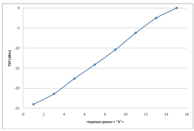
Figure 3: BLE113 TX power as a function of the setting in the HW configuration file
