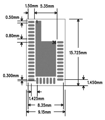
Figure 7: Physical dimensions and pinout (top view)
