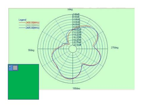
Figure 4: Radiation pattern of BLE113, top view
