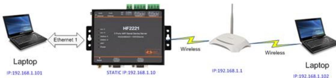
Figure 23. Ethernet Port Function1 (Bridge)
