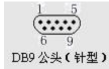
Figure 3. RS232 Pin Definition(Male/Needle Type)
