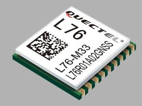
L76, the smallest GNSS module, is a single receiver module integrated GLONASS with GPS system. It provides simultaneous GPS and Compass GLONASS open service L1 reception capability. With 33 tracking channels, 99 acquisition channels, and 210 PRN channels, L76 can acquire and track any mix of GPS and GLONASS signals.
