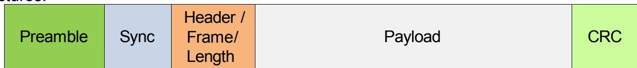
Figure 12. Packet Handler Structure
