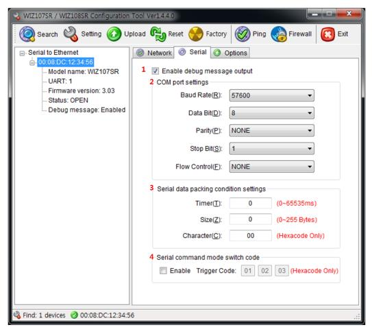
Figure 7. WIZ107SR Configuration Tool (Serial Configuration Page)
