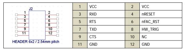
Figure 2. WIZ107SR Connector Pin Assignment
