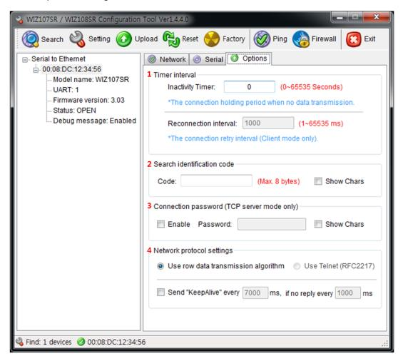
Figure 8. WIZ107SR Configuration Tool (Option Configuration Page)
