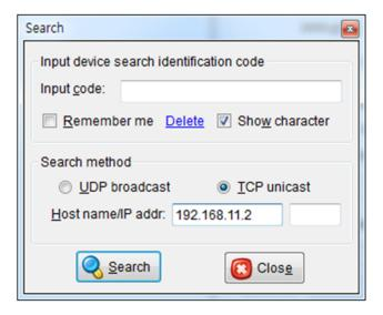
Figure 5. Searching with TCP unicast method
