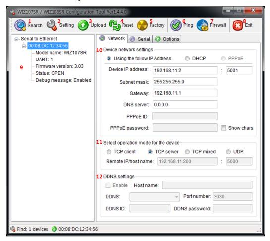
Figure 3. WIZ107SR Configuration Tool (Network Configuration Page)
