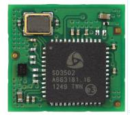
The ZM5202 module combines a Z-Wave<sup>®</sup> SD3502 SoC (with a built-in microcontroller and Z-Wave RF transceiver), crystal, and passive RF components. This makes the ZM5202 ideal for single microcontroller
