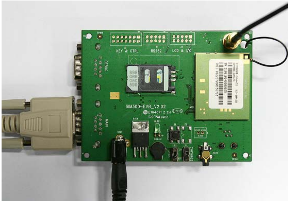
Figure 2: Top view of SIM900B EVB
