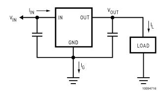
FIGURE 6. Power Dissipation Diagram
