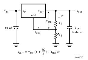
FIGURE 2. Basic Adjustable Regulator
