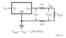
FIGURE 3. Typical Application using Fixed Output Regulator
