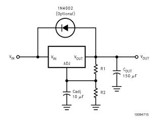
FIGURE 5. Regulator with Protection Diode
