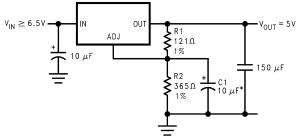
\*C1 IMPROVES RIPPLE REJECTION.  $X_C$  SHOULD BE  $\approx$  R1 AT RIPPLE FREQUENCY
