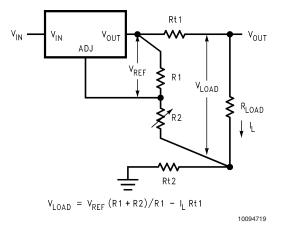
FIGURE 4. Best Load Regulation using Adjustable Output Regulator
