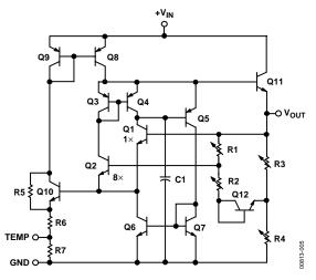
Figure 5. Schematic Diagram
