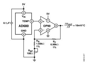
Figure 17. Differential Temperature Transducer
