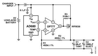
Figure 20. Voltage Regulator for Portable Equipment
