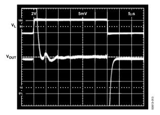
Figure 13. Output Response with Capacitive Load
