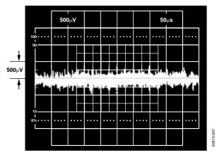
Figure 7. Broadband Noise at 300 kHz
