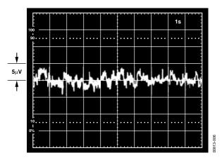
Figure 6. 0.1 Hz to 10 Hz Noise
