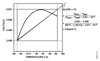
Figure 15. Typical AD680AN/AD680AR Temperature Drift
