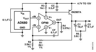
Figure 19. 4.5 V Reference Running from a Single 5 V Supply
