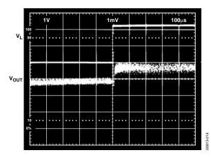
Figure 14. Typical Load Regulation Characteristics
