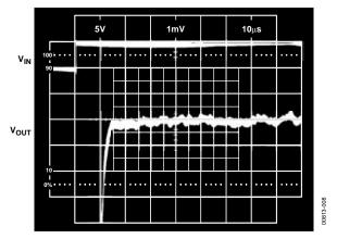
Figure 8. Turn-On Settling Time
