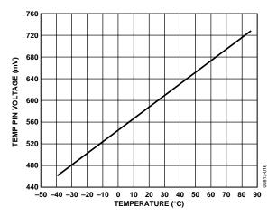
Figure 16. TEMP Pin Transfer Characteristics
