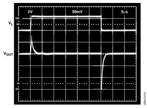
Figure 10. Large Scale Transient Response
