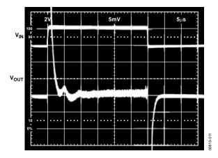
Figure 11. Fine Scale Settling for Transient Load
