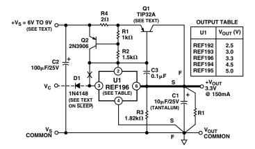
Figure 4. A Boosted 3.3 V Reference with Current Limiting
