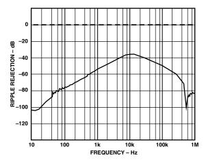
TPC 7a. Ripple Rejection vs. Frequency
