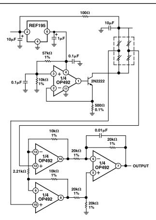
Figure 12. A Low Power, Strain Gage Circuit
