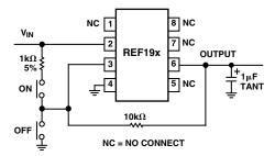
Figure 3. Membrane Switch Controlled Power Supply
