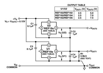
Figure 6. Stacking Voltage References with the REF19x
