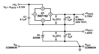
Figure 7. Stacking Voltage References with the REF19x
