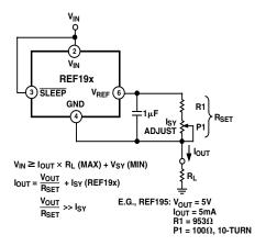
Figure 8. A Low Dropout, Precision Current Source
