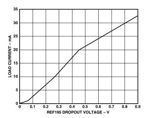
TPC 13. Load Current vs. Dropout Voltage
