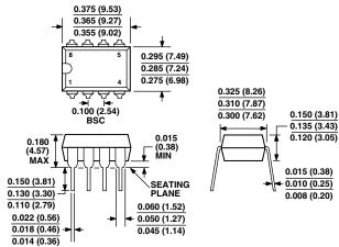
**COMPLIANT TO JEDEC STANDARDS MO-095AA** CONTROLLING DIMENSIONS ARE IN INCHES; MILLIMETER DIMENSIONS (IN PARENTHESES) ARE ROUNDED-OFF INCH EQUIVALENTS FOR REFERENCE ONLY AND ARE NOT APPROPRIATE FOR USE IN DESIGN
