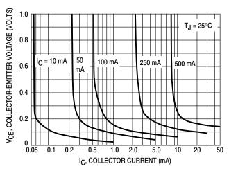
Figure 5. Collector Saturation Region
