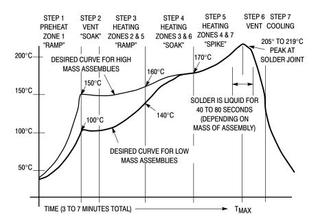
Figure 7. Typical Solder Heating Profile
