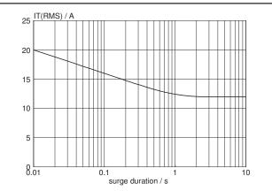
Fig.5. Maximum permissible repetitive rms on-state current  $I_{T(RMS)}$ , versus surge duration, for sinusoidal currents, f = 50 Hz;  $T_{mb} \le 109 ^{\circ}\text{C}$ .
