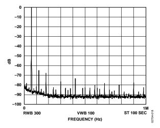
Figure 18.  $f_{MCLK} = 25$  MHz,  $f_{OUT} = 60$  kHz, Frequency Word = 0x009D495
