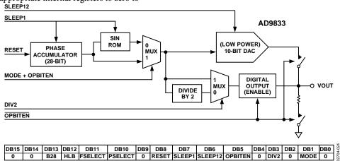
Figure 24. Function of Control Bits
