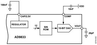
Figure 2. Test Circuit Used to Test Specifications
