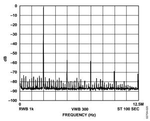
Figure 20.  $f_{MCLK} = 25$  MHz,  $f_{OUT} = 2.4$  MHz, Frequency Word = 0x189374D
