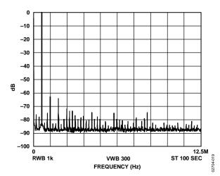
Figure 19.  $f_{MCLK} = 25$  MHz,  $f_{OUT} = 600$  kHz, Frequency Word = 0x0624DD3
