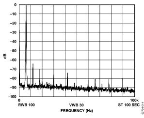
Figure 14.  $f_{MCLK} = 10$  MHz,  $f_{OUT} = 2.4$  kHz, Frequency Word = 0x000FBA9
