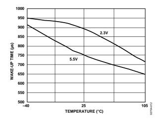
Figure 12. Wake-Up Time vs. Temperature
