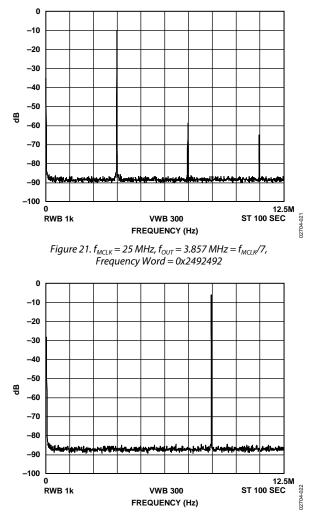
Figure 22.  $f_{MCLK} = 25 \text{ MHz}, f_{OUT} = 8.333 \text{ MHz} = f_{MCLK}/3,$ Frequency Word = 0x5555555
