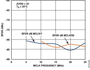
Figure 8. Narrow-Band SFDR vs. MCLK Frequency
