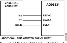
Figure 29. ADSP-2101/ADSP-2103 to AD9833 Interface
