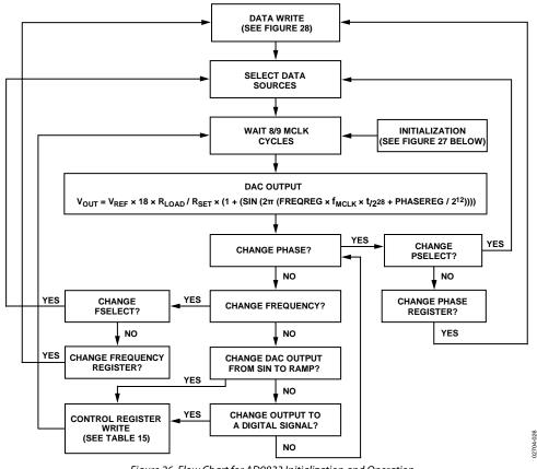
Figure 26. Flow Chart for AD9833 Initialization and Operation
