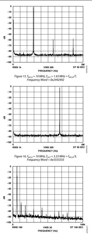
Figure 17.  $f_{MCLK} = 25 \text{ MHz}$ ,  $f_{OUT} = 6 \text{ kHz}$ , Frequency Word = 0x000FBA9
