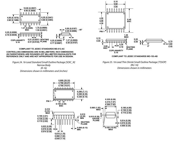
COMPLIANT TO JEDEC STANDARDS MS-001-AB CONTROLLING DIMENSIONS ARE IN INCHES; MILLIMETER DIMENSIONS (IN PARENTHESES) ARE ROUNDED-OFF INCH EQUIVALENTS FOR REFERENCE ONLY AND ARE NOT APPROPRIATE FOR USE IN DESIGN. CORNER LEADS MAY BE CONFIGURED AS WHOLE OR HALF LEADS.
