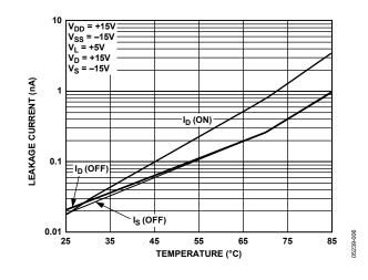
Figure 8. Leakage Currents as a Function of Temperature
