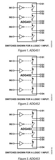
The ADG453 has two switches with digital control logic similar to that of the ADG451, while the logic is inverted on the other two switches.
