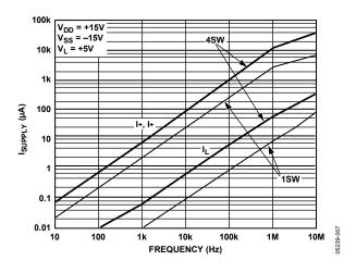
Figure 9. Supply Current vs. Input Switching Frequency
