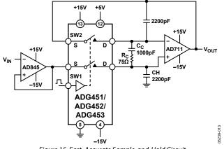
Figure 15. Fast, Accurate Sample-and-Hold Circuit
