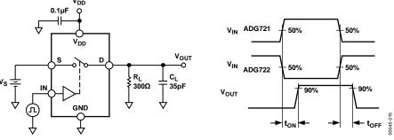
Figure 15. Switching Times
