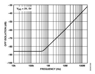
Figure 9. Off Isolation vs. Frequency
