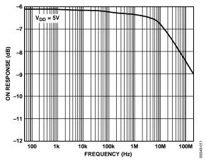
Figure 11. On Response vs. Frequency
