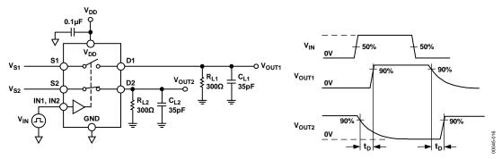
Figure 16. Break-Before-Make Time Delay, t<sub>D</sub> (ADG723 Only)
