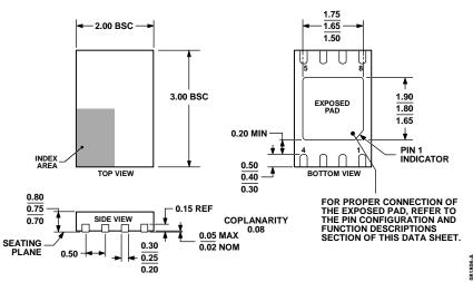
Figure 24. 8-Lead Lead Frame Chip Scale Package [LFCSP\_WD] 3 mm × 2 mm Body, Very Very Thin, Dual Lead (CP-8-4) Dimensions shown in millimeters
