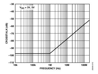
Figure 10. Crosstalk vs. Frequency
