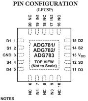
1. NC = NO CONNECT. 2. EXPOSED PAD TIED TO SUBSTRATE, GND.
