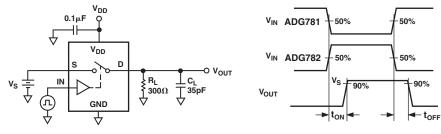
Test Circuit 4. Switching Times
