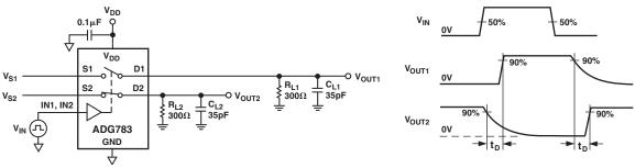
Test Circuit 5. Break-Before-Make Time Delay, t<sub>D</sub>
