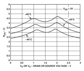
TPC 2. On Resistance as a Function of  $V_D$  ( $V_S$ ) for Different Temperatures  $V_{DD} = 3 V$
