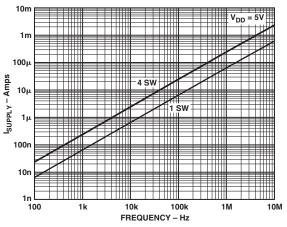
TPC 4. Supply Current vs. Input Switching Frequency
