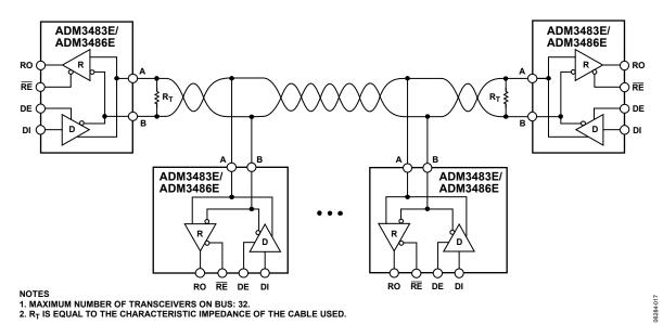
Figure 31. ADM3483E/ADM3486E Typical Half-Duplex RS-485 Network
