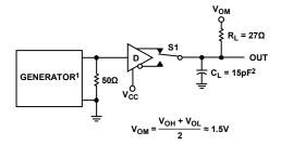
$^{1}\text{PPR}$  = 250kHz, 50% DUTY CYCLE,  $t_{R} \leq$  6.0ns,  $Z_{O}$  = 50 $\Omega$ .  $^{2}C_{L}$  INCLUDES PROBE AND STRAY CAPACITANCE.
