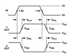
Figure 11. Driver Propagation Delays
