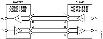
Figure 32. ADM3488E/ADM3490E Full-Duplex Point-to-Point Applications
