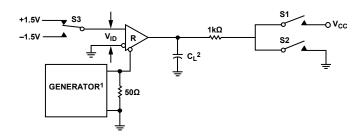
^1PPR = 250kHz, 50% DUTY CYCLE,  $t_R \le$  6.0ns,  $Z_O$  = 50 $\Omega$ .  $^2C_L$  INCLUDES PROBE AND STRAY CAPACITANCE.
