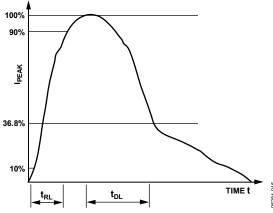
Figure 30. Human Body Model and Current Waveform
