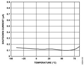
Figure 25. Shutdown Current vs. Temperature
