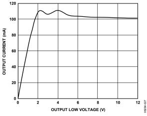
Figure 22. Output Current vs. Driver Output Low Voltage
