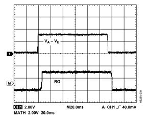
Figure 29. ADM3483E/ADM3488E Receiver Propagation Delay
