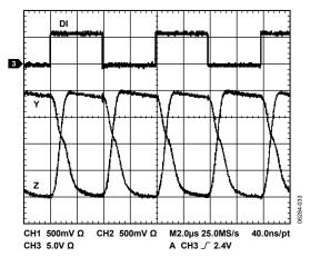
Figure 28. ADM3483E/ADM3488E Driver Propagation Delay
