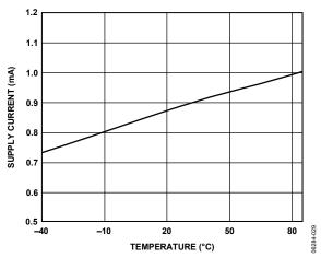
Figure 24. Supply Current vs. Temperature
