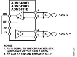
Figure 34. Line Repeater for ADM3488E/ADM3490E/ADM3491E
