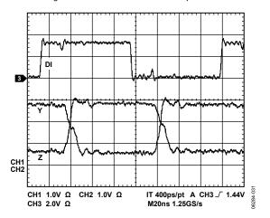
Figure 26. ADM3490E/ADM3491E Driver Propagation Delay
