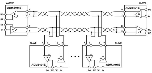
NOTES 1. MAXIMUM NUMBER OF NODES: 32. 2.  $R_{\rm T}$  IS EQUAL TO THE CHARACTERISTIC IMPEDANCE OF THE CABLE USED.
