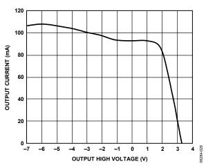
Figure 23. Output Current vs. Driver Output High Voltage
