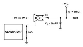
$^{1}\text{PPR}$  = 250kHz, 50% DUTY CYCLE,  $t_{R}$   $\leq$  6.0ns,  $z_{O}$  = 50  $\!\Omega$ .  $^{2}C_{L}$  INCLUDES PROBE AND STRAY CAPACITANCE.
