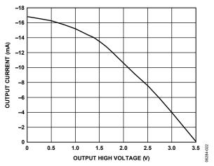
Figure 17. Output Current vs. Receiver Output High Voltage
