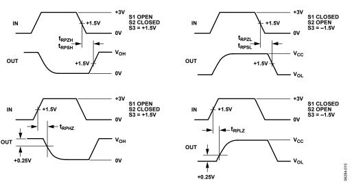
Figure 15. Receiver Enable and Disable Times
