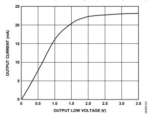
Figure 16. Output Current vs. Receiver Output Low Voltage
