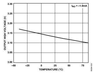
Figure 18. Receiver Output High Voltage vs. Temperature
