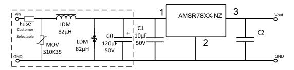
C1: A low ESR capacitor is required to keep the noise of the converter to a minimum.
