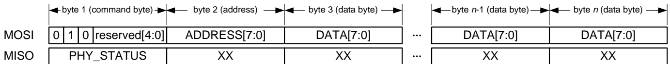
Figure 6-12. Packet Structure – SRAM Write Access.
