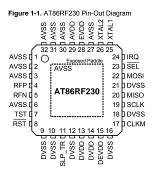
**Note:** The exposed paddle is electrically connected to the die inside the package. It shall be soldered to the board to ensure electrical and thermal contact and good mechanical stability.
