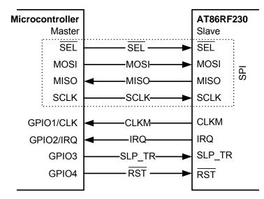
Microcontrollers with a master SPI, such as Atmel's AVR family, interface directly to the AT86RF230. The SPI is used for Frame Buffer and register access. The additional control signals are connected to the GPIO/IRQ interface of the microcontroller. Table 6-1 introduces the radio transceiver I/O signals and their functionality.
