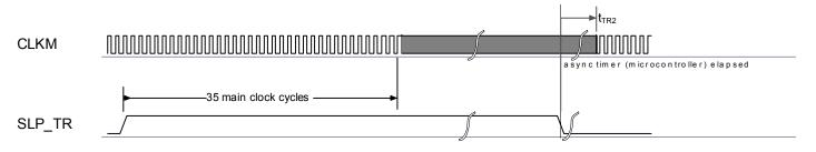
For synchronous systems, where CLKM is used as a microcontroller clock source and the SPI master clock (SCLK) is directly derived from CLKM, the AT86RF230 supports an additional power-down mode for receive operating states RX\_ON and RX\_AACK\_ON.
