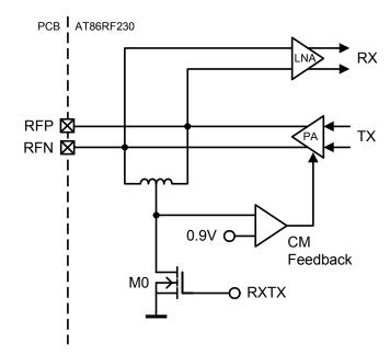
RF port DC values depend on the operating mode. In TRX\_OFF state (see section 7.1.2), when the analog front end is disabled, the RF pins are pulled to ground, preventing a floating voltage.
