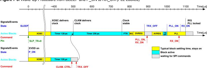
Figure 7-3. Wake-Up Procedure from SLEEP and P\_ON to RX\_ON (PLL Locked)
