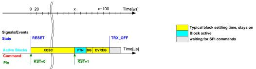
Figure 7-4. Reset Procedure
