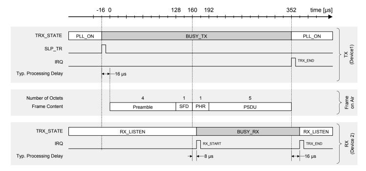
Figure 7-2. Timing of RX\_START and TRX\_END Interrupts in Basic Operating Mode (see register 0x0F)
