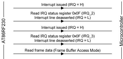
Critical protocol timing could require starting the frame upload as soon as possible. The first byte of the frame data can be read 32 µs after the IRQ\_2 (RX\_START) interrupt. The microcontroller must ensure to read slower than the frame is received. Otherwise, the Frame Buffer wills under run, IRQ\_6 (TRX\_UR) interrupt is issued. The frame data are not valid anymore and need to read again. The LQI byte can be uploaded to the microcontroller after the IRQ\_3 (TRX\_END) interrupt was issued.
