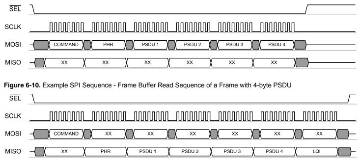
Access violations during a Frame Buffer write or read access are indicated by a TRX\_UR interrupt. For further details refer to section 9.3.3.
