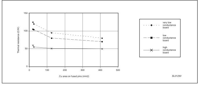
Figure 6. SO-14 Thermal Resistance vs. PCB Configuration, Note 1, 2, 3
