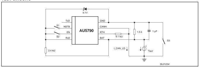
Loss of ground test circuit Figure 3.
