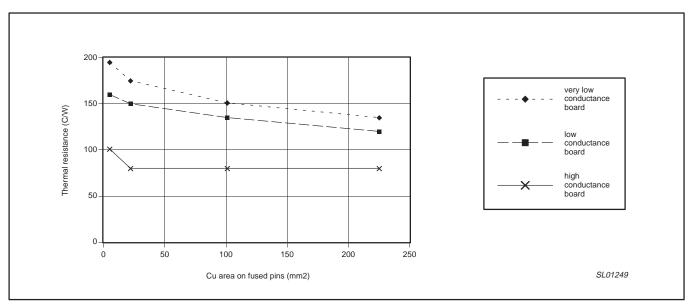
Figure 5. SO-8 Thermal Resistance vs. PCB Configuration, Note 1, 2, 3
