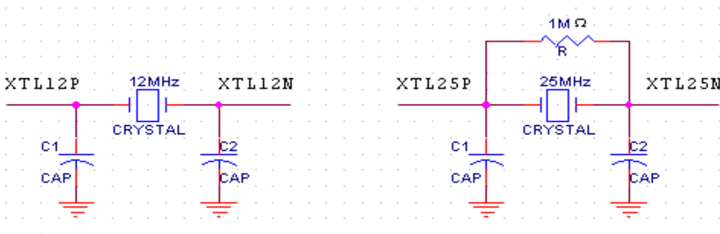
Figure 20 : One external 1M ohm resistor on 25MHz crystal oscillator is necessary
