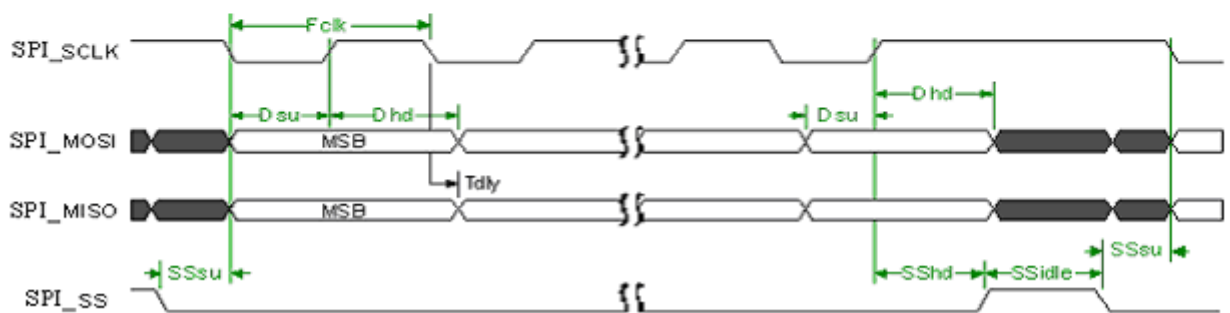
SPI Slave Mode Timing Diagram in Mode 3
