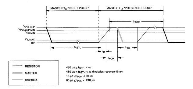
In order not to mask interrupt signaling by other devices on the 1-Wire bus,  $t_{RSTL} + t_R$  should always be less than 960 $\mu$ s.
