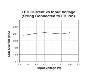
The feedback loop tightly regulates the current in the branch connected to FB pin, while the current in the other branch depends on the sum of the LED's forward voltages,  $V_{OUT}$  and the ballast resistor. The input and the output ripple is less than  $3mV_{BMS}$ , for load currents up to 40mA.
