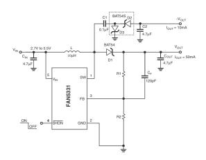
Figure 7. Dual (±) Boost Converter
