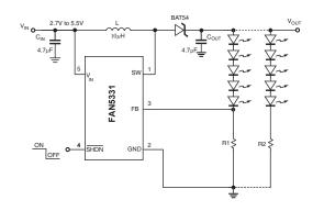
Figure 6. Low Noise Boost LED Driver
