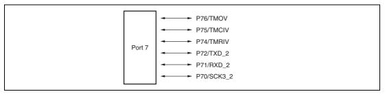
Figure 9.6 Port 7 Pin Configuration
