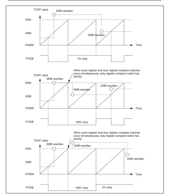
Figure 13.24 Example of PWM Mode Operation (3)
