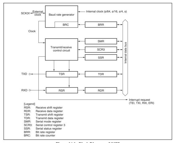
Figure 16.1 Block Diagram of SCI3
