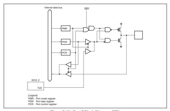
Figure B.19 Port 7 Block Diagram (P72)
