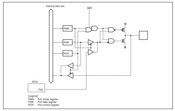
Figure B.8 Port 2 Block Diagram (P22)
