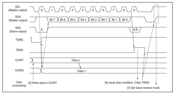
Figure 17.6 Master Transmit Mode Operation Timing (2)
