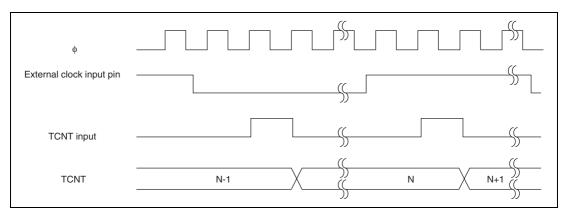
Figure 13.11 Count Timing at External Clock Operation (Both Edges Detected)
