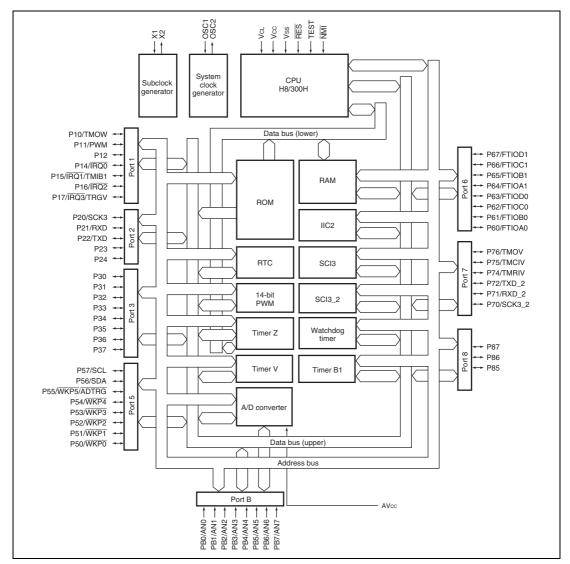
Figure 1.1 Internal Block Diagram of H8/3687 Group of F-ZTAT<sup>™</sup> and Mask-ROM Versions
