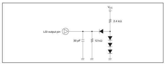
Figure 23.8 Output Load Circuit
