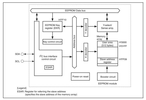
Figure 19.1 Block Diagram of EEPROM
