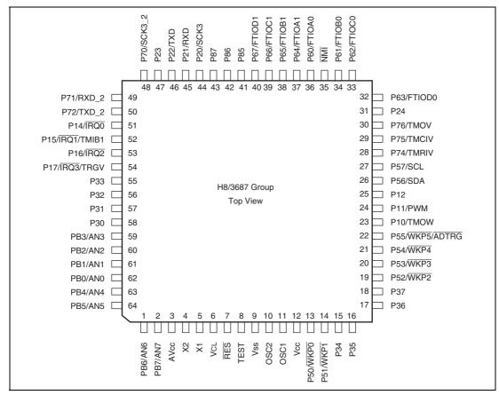
Figure 1.3 Pin Arrangement of H8/3687 Group of F-ZTAT<sup>™</sup> and Mask-ROM Versions (FP-64E, FP-64A)
