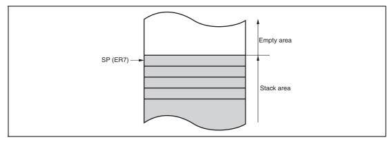
Figure 2.4 Relationship between Stack Pointer and Stack Area
