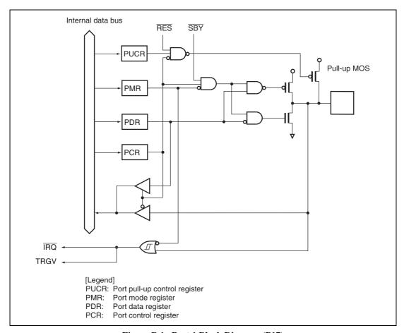
Figure B.1 Port 1 Block Diagram (P17)
