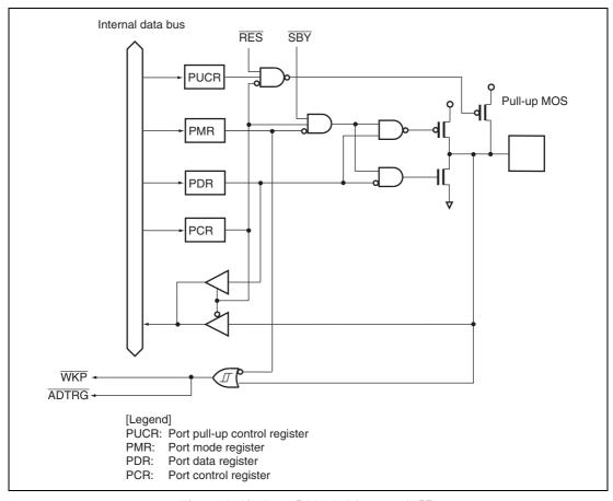
Figure B.13 Port 5 Block Diagram (P55)
