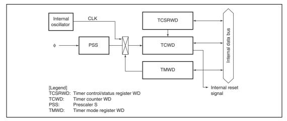
Figure 14.1 Block Diagram of Watchdog Timer
