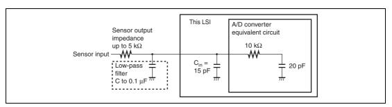
Figure 18.6 Analog Input Circuit Example
