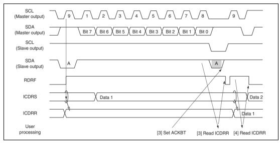
Figure 17.12 Slave Receive Mode Operation Timing (2)
