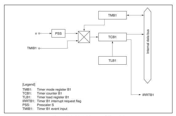
Figure 11.1 Block Diagram of Timer B1
