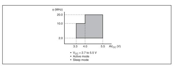
Range of Power Supply Voltage and Oscillation Frequency when Low-Voltage Detection Circuit is Used
