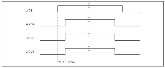
Figure 20.5 Timing for Operation/Release of Low-Voltage Detection Circuit
