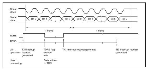
Figure 16.10 Example of SCI3 Transmission in Clocked Synchronous Mode
