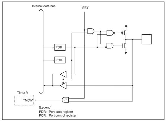
Figure B.17 Port 7 Block Diagram (P75)
