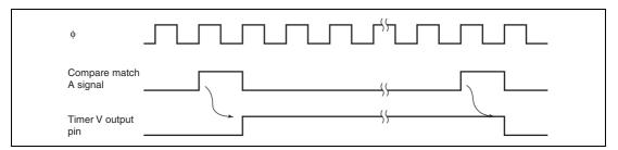
Figure 12.6 TMOV Output Timing
