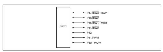
Figure 9.1 Port 1 Pin Configuration
