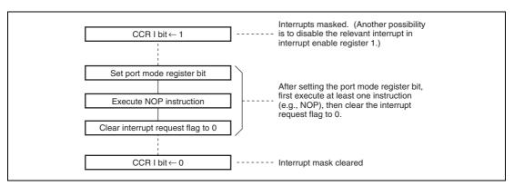
Figure 3.4 Port Mode Register Setting and Interrupt Request Flag Clearing Procedure
