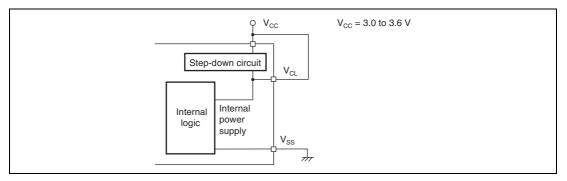
Figure 21.2 Power Supply Connection when Internal Step-Down Circuit is Not Used
