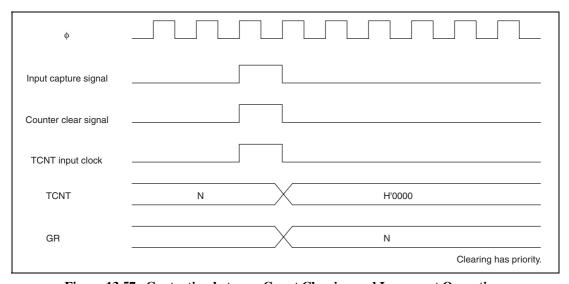
Figure 13.57 Contention between Count Clearing and Increment Operations by Input Capture
