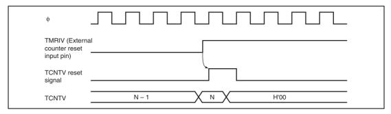
Figure 12.8 Clear Timing by TMRIV Input
