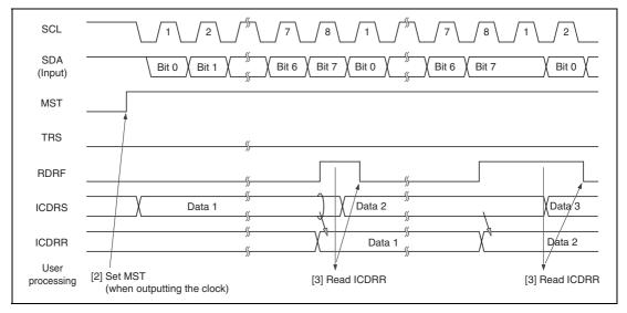
Figure 17.15 Receive Mode Operation Timing
