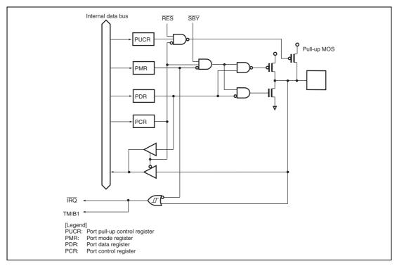
Figure B.3 Port 1 Block Diagram (P15)
