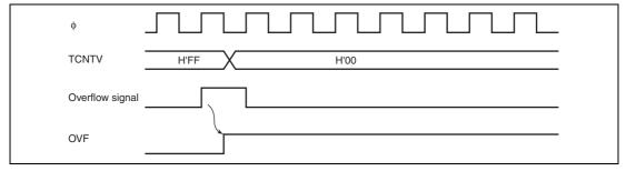
Figure 12.4 OVF Set Timing
