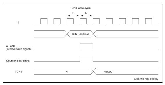
Figure 13.52 Contention between TCNT Write and Clear Operations
