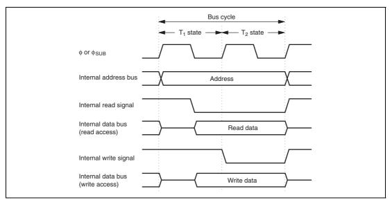
Figure 2.9 On-Chip Memory Access Cycle
