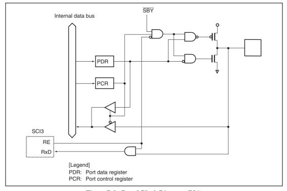
Figure B.9 Port 2 Block Diagram (P21)
