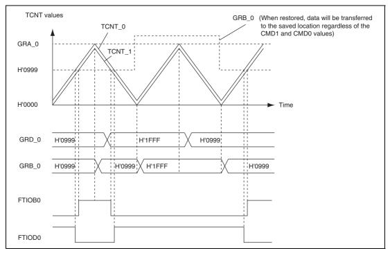
$Figure \ 13.42 \quad Buffer \ Operation \ (3)$  (Buffer Operation in Complementary PWM Mode CMD1 = CMD0 = 1)
