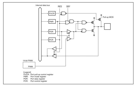
Figure B.5 Port 2 Block Diagram (P11)
