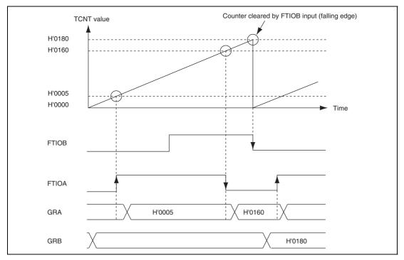
Figure 13.17 Example of Input Capture Operation
