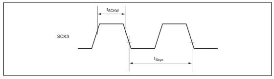
Figure 23.5 SCK3 Input Clock Timing
