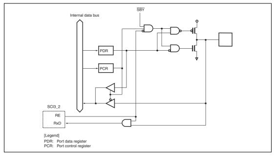
Figure B.20 Port 7 Block Diagram (P71)
