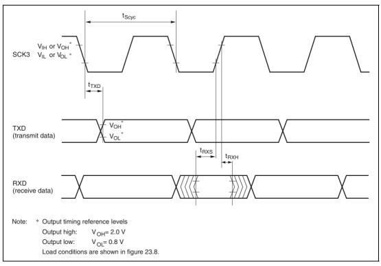
Figure 23.6 SCI Input/Output Timing in Clocked Synchronous Mode
