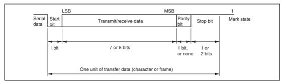
Figure 16.2 Data Format in Asynchronous Communication
