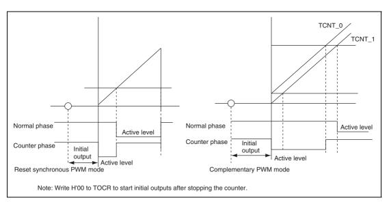
Figure 13.4 Example of Outputs in Reset Synchronous PWM Mode and Complementary PWM Mode
