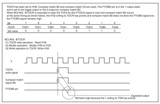
Figure 13.59 When Compare Match and Bit Manipulation Instruction to TOCR
