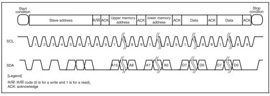
Figure 19.2 EEPROM Bus Format and Bus Timing
