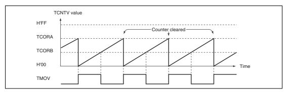
Figure 12.9 Pulse Output Example
