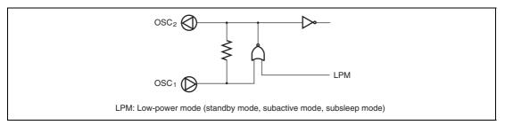
Figure 5.2 Block Diagram of System Clock Generator
