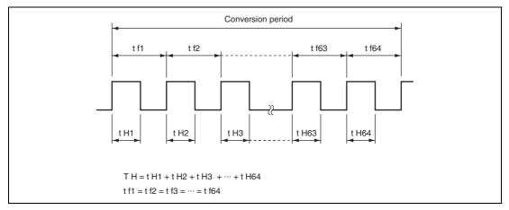
Figure 15.2 Waveform Output by 14-Bit PWM
