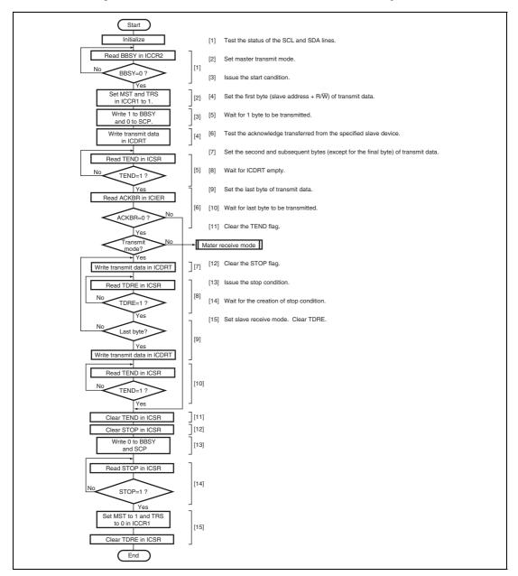
Figure 17.17 Sample Flowchart for Master Transmit Mode
