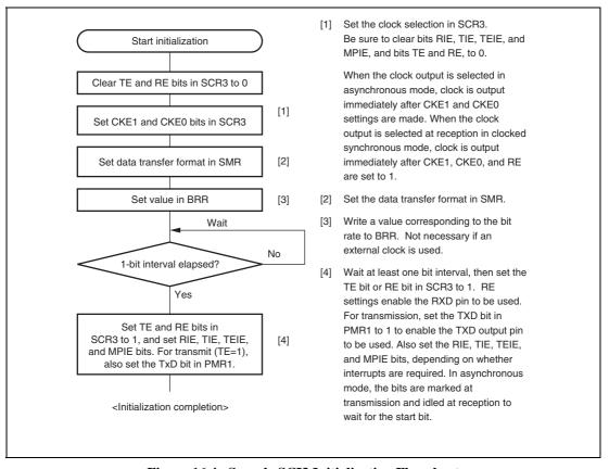
Figure 16.4 Sample SCI3 Initialization Flowchart
