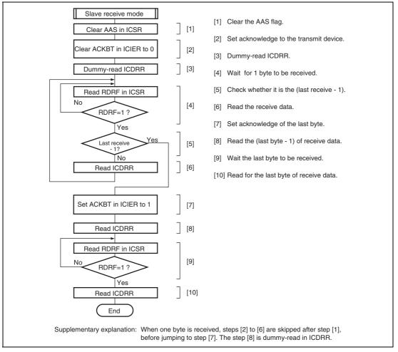
Figure 17.20 Sample Flowchart for Slave Receive Mode
