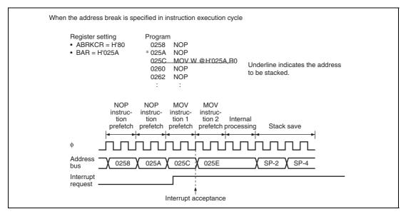
Figure 4.2 Address Break Interrupt Operation Example (1)
