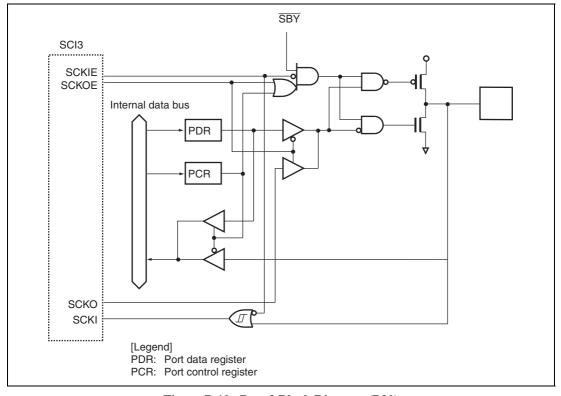
Figure B.10 Port 2 Block Diagram (P20)
