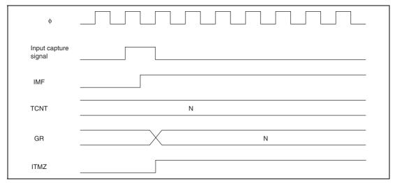
Figure 13.49 IMF Flag Set Timing at Input Capture
