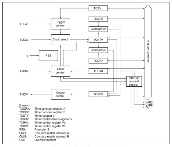
Figure 12.1 Block Diagram of Timer V
