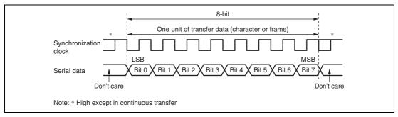
Figure 16.9 Data Format in Clocked Synchronous Communication
