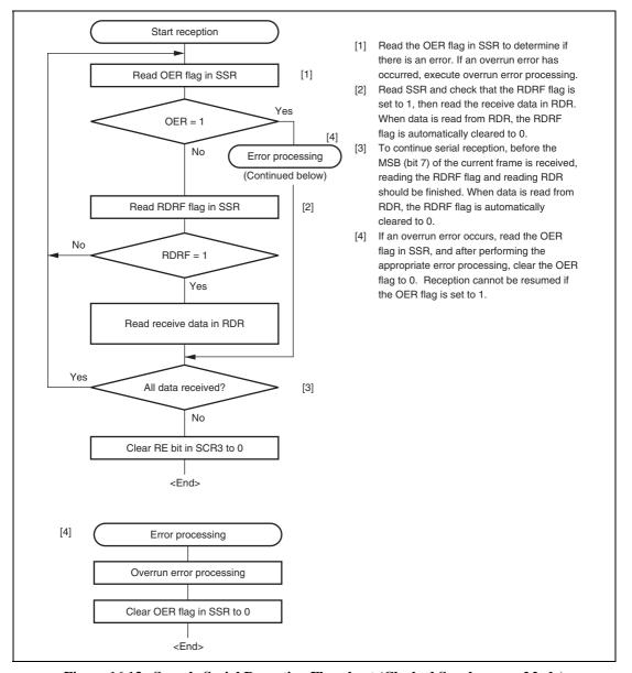
Figure 16.13 Sample Serial Reception Flowchart (Clocked Synchronous Mode)
