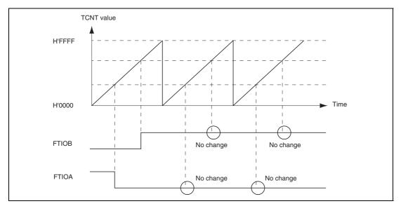
Figure 13.13 Example of 0 Output/1 Output Operation
