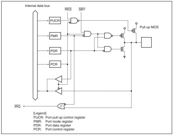
Figure B.2 Port 1 Block Diagram (P14, P16)
