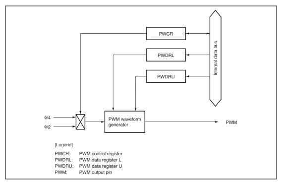
Figure 15.1 Block Diagram of 14-Bit PWM
