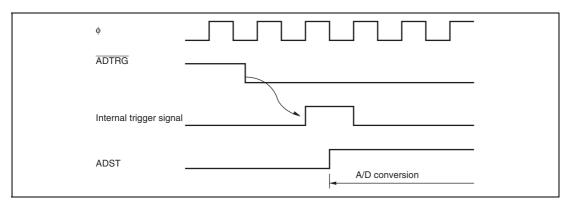
Figure 18.3 External Trigger Input Timing
