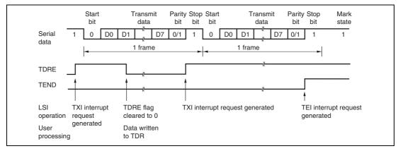
Figure 16.5 Example of SCI3 Transmission in Asynchronous Mode (8-Bit Data, Parity, One Stop Bit)
