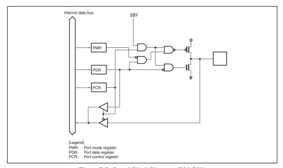
Figure B.7 Port 2 Block Diagram (P24, P23)
