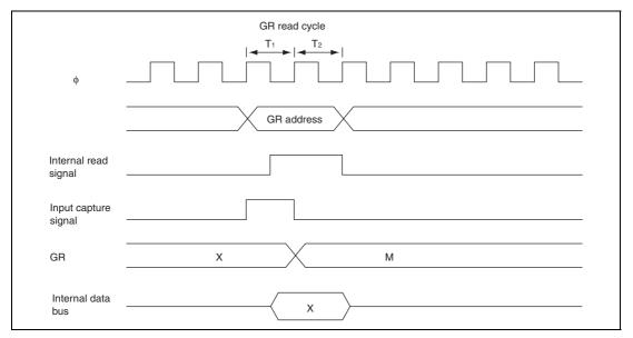
Figure 13.56 Contention between GR Read and Input Capture
