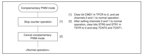
Figure 13.30 Canceling Procedure of Complementary PWM Mode
