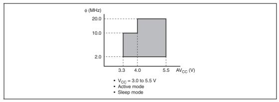
Range of Power Supply Voltage and Oscillation Frequency when Low-Voltage Detection Circuit is Used
