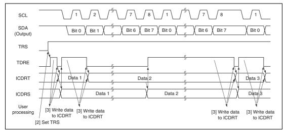
Figure 17.14 Transmit Mode Operation Timing
