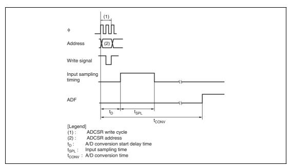
Figure 18.2 A/D Conversion Timing
