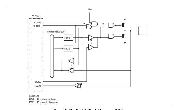
Figure B.21 Port 7 Block Diagram (P70)
