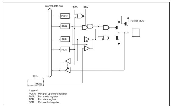
Figure B.6 Port 1 Block Diagram (P10)
