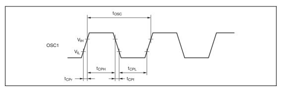
Figure 23.1 System Clock Input Timing
