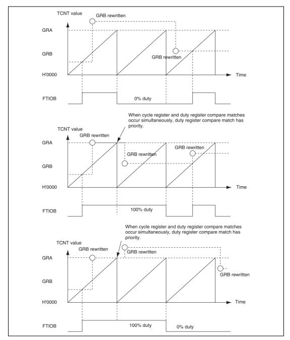
Figure 13.25 Example of PWM Mode Operation (4)
