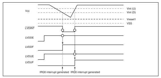
Figure 20.4 Operational Timing of LVDI Circuit
