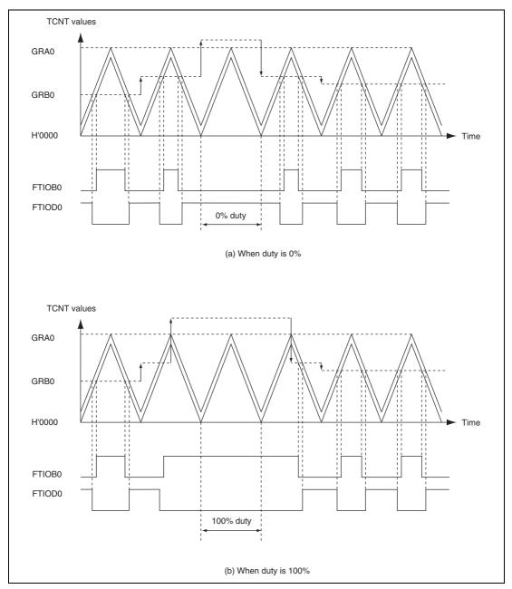
Figure 13.32 (2) Example of Complementary PWM Mode Operation (TPSC2 = TPSC1 = TPSC0  $\neq$  0) (3)
