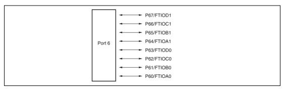
Figure 9.5 Port 6 Pin Configuration
