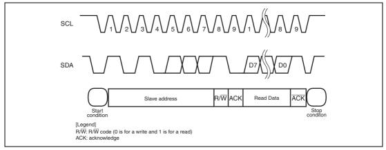
Figure 19.5 Current Address Read Operation
