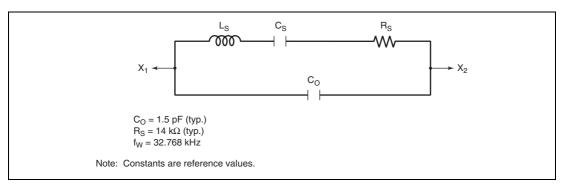
Figure 5.9 Equivalent Circuit of 32.768-kHz Crystal Resonator
