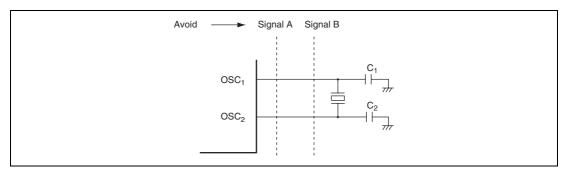
Figure 5.11 Example of Incorrect Board Design
