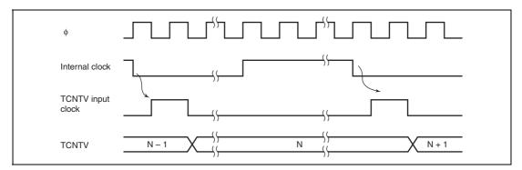
Figure 12.2 Increment Timing with Internal Clock
