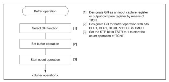
Figure 13.37 Example of Buffer Operation Setting Procedure
