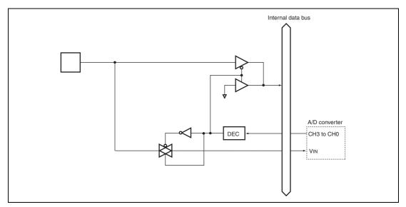
Figure B.23 Port B Block Diagram (PB7 to PB0)
