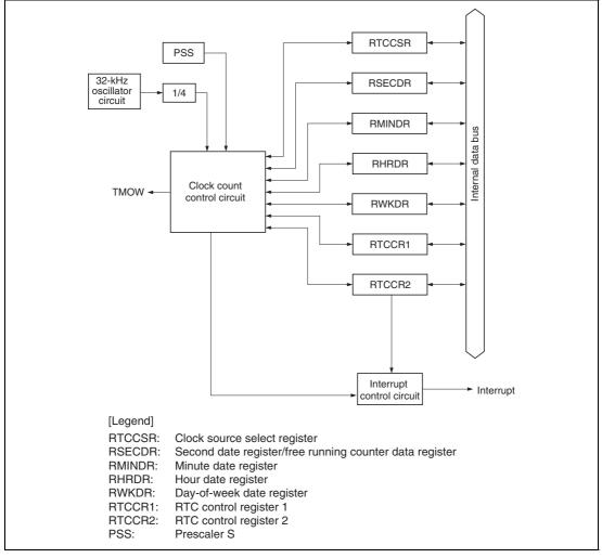
Figure 10.1 Block Diagram of RTC
