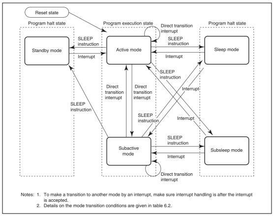
Figure 6.1 Mode Transition Diagram
