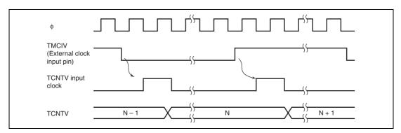
Figure 12.3 Increment Timing with External Clock
