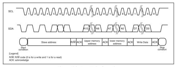
Figure 19.3 Byte Write Operation
