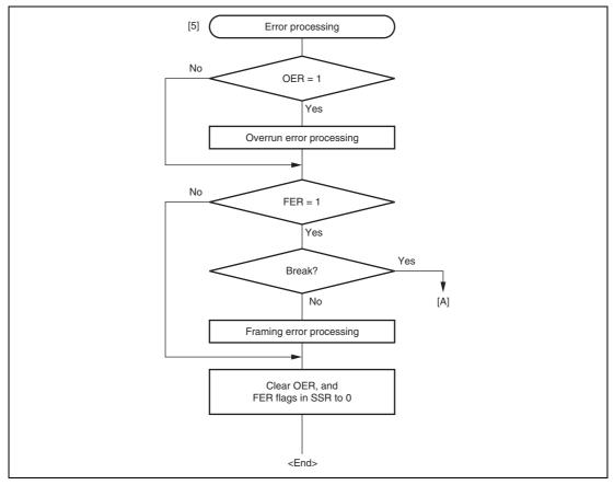
Figure 16.17 Sample Multiprocessor Serial Reception Flowchart (2)
