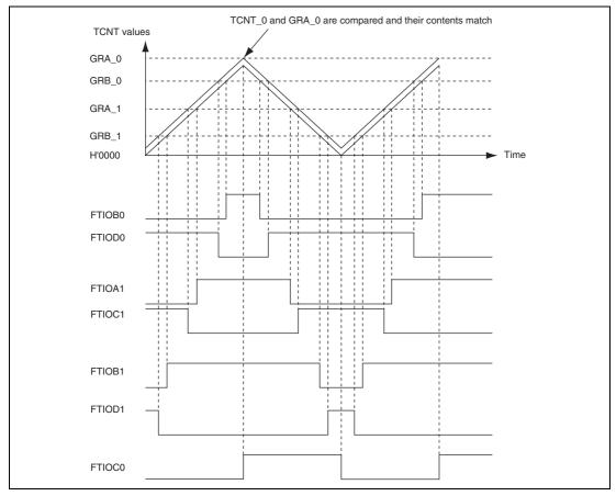
Figure 13.31 Example of Complementary PWM Mode Operation (1)
