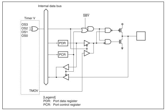
Figure B.16 Port 7 Block Diagram (P76)
