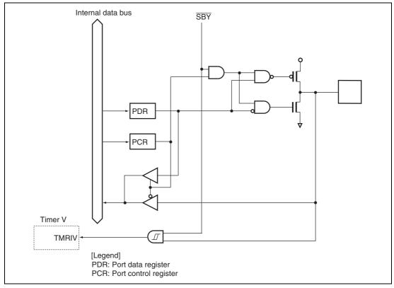
Figure B.18 Port 7 Block Diagram (P74)
