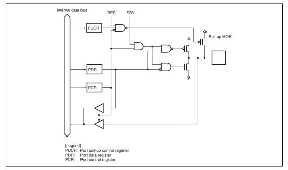
Figure B.4 Port 1 Block Diagram (P12)
