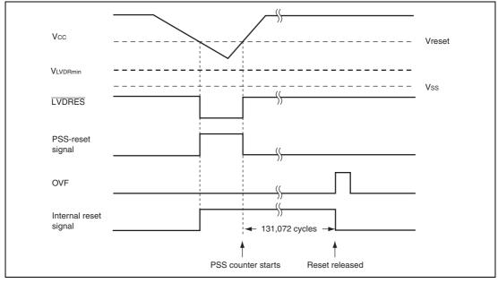
Figure 20.3 Operational Timing of LVDR Circuit
