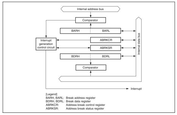
Figure 4.1 Block Diagram of Address Break
