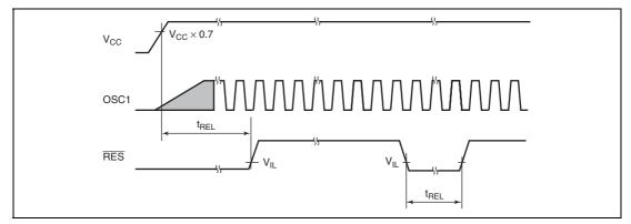
Figure 23.2 RES Low Width Timing
