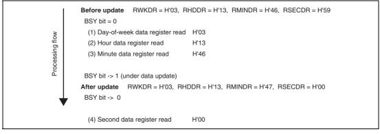
Figure 10.4 Example: Reading of Inaccurate Time Data
