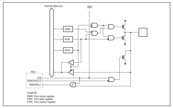
Figure B.12 Port 5 Block Diagram (P57, P56)\*
