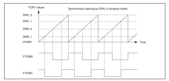
Figure 13.20 Example of Synchronous Operation
