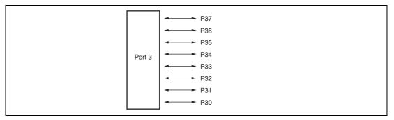
Figure 9.3 Port 3 Pin Configuration
