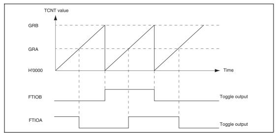
Figure 13.14 Example of Toggle Output Operation
