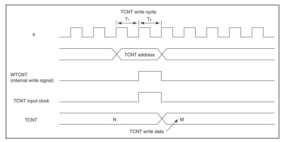
Figure 13.53 Contention between TCNT Write and Increment Operations
