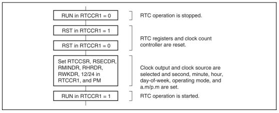
Figure 10.3 Initial Setting Procedure
