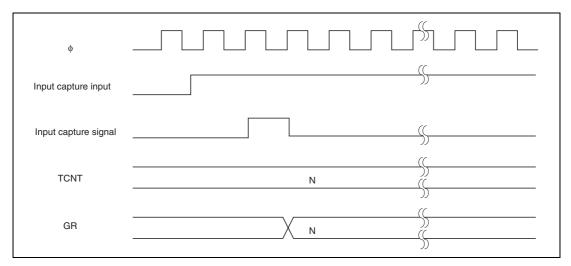
Figure 13.18 Input Capture Signal Timing
