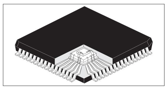
Figure E.1 EEPROM Stacked-Structure Cross-Sectional View
