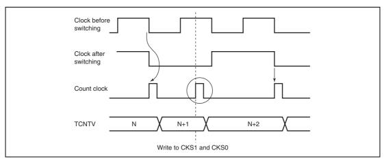
Figure 12.13 Internal Clock Switching and TCNTV Operation
