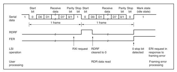
Figure 16.7 Example of SCI3 Reception in Asynchronous Mode (8-Bit Data, Parity, One Stop Bit)
