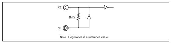
Figure 5.7 Block Diagram of Subclock Generator
