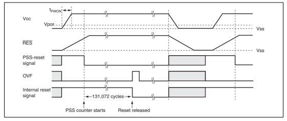
Figure 20.2 Operational Timing of Power-On Reset Circuit
