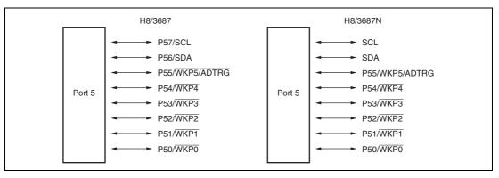
Figure 9.4 Port 5 Pin Configuration
