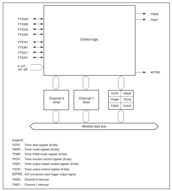
Figure 13.1 Timer Z Block Diagram
