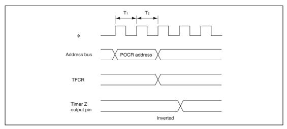
Figure 13.47 Example of Output Inverse Timing of Timer Z by Writing to POCR
