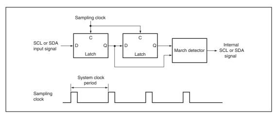
Figure 17.16 Block Diagram of Noise Conceler
