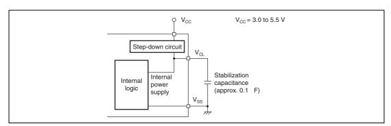
Figure 21.1 Power Supply Connection when Internal Step-Down Circuit is Used
