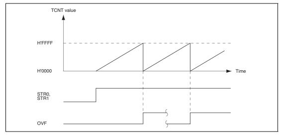
Figure 13.8 Free-Running Counter Operation
