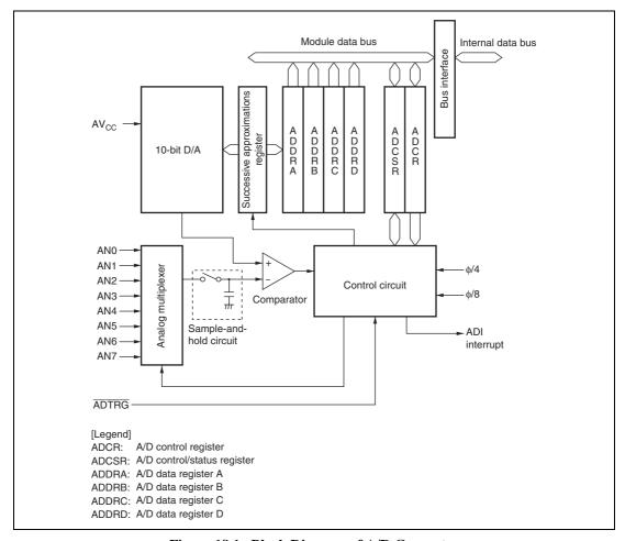
Figure 18.1 Block Diagram of A/D Converter
