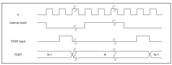
Figure 13.10 Count Timing at Internal Clock Operation
