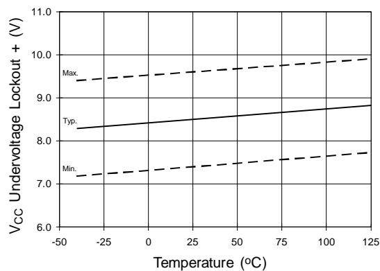
Figure 24. V<sub>CC</sub> Undervoltage (+) vs. Temperature
