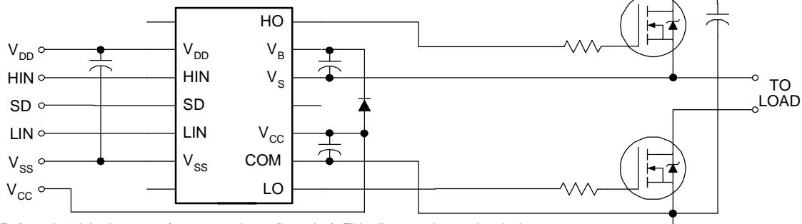
(Refer to Lead Assignments for correct pin configuration). This diagram shows electrical connections only. Please refer to our Application Notes and DesignTips for proper circuit board layout.
