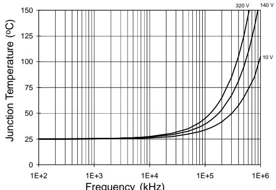
**Figure 31. IRS2110/IRS2113  $T_J$  vs. Frequency
