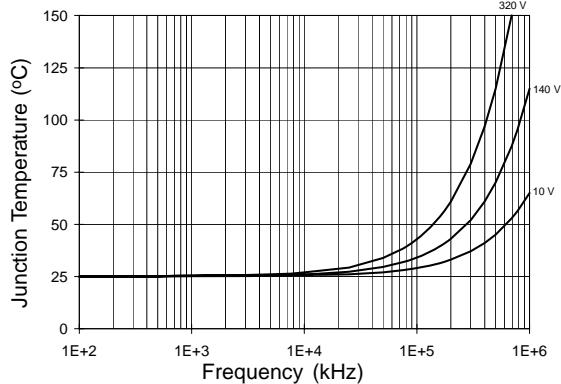
**Figure 29. IRS2110/IRS2113  $T_J$  vs. Frequency
