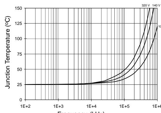
**Figure 34. IRS2110S/IRS2113S  $T_J$  vs. Frequency
