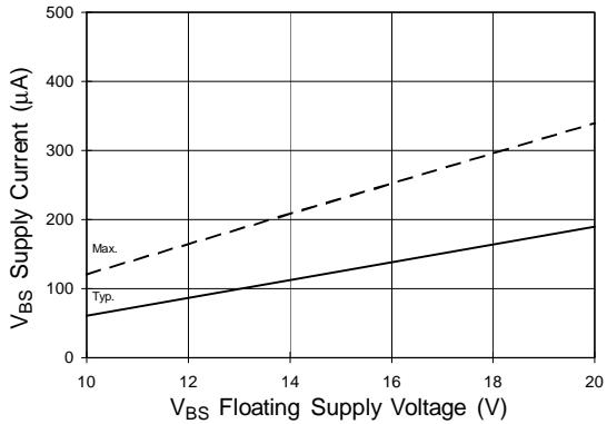
Figure 17B. V<sub>BS</sub> Supply Current vs. Voltage
