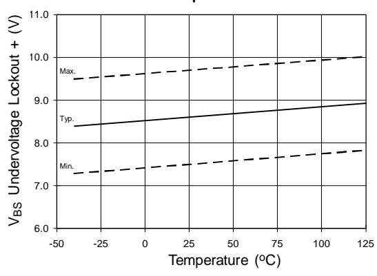
Figure 22. V<sub>BS</sub> Undervoltage (+) vs. Temperature
