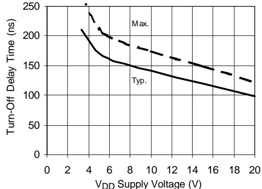
Figure 8C. Turn-Off Time vs. V<sub>DD</sub> Supply Voltage
