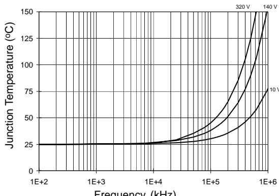
**Figure 32. IRS2110S/IRS2113S  $T_J$  vs. Frequency
