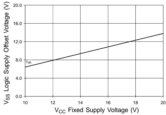
Figure 37. Maximum V<sub>SS</sub> Positive Offset vs.
