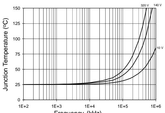
**Figure 33. IRS2110S/IRS2113S  $T_J$  vs. Frequency
