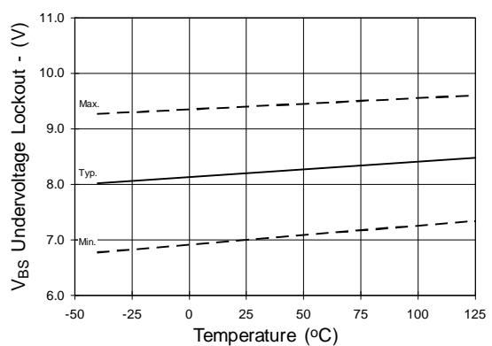
Figure 23. V<sub>BS</sub> Undervoltage (-) vs. Temperature
