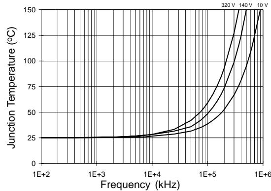
Figure 35. IRS2110S/IRS2113S T<sub>J</sub> vs. Frequency
