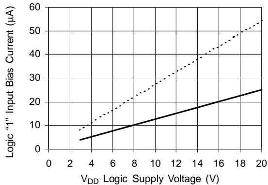
Figure 20B. Logic "1" Input Current vs. V<sub>DD</sub> Voltage
