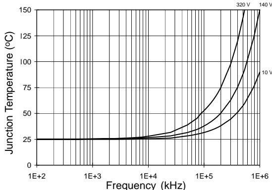
**Figure 30. IRS2110/IRS2113  $T_J$  vs. Frequency
