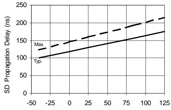
Figure 9A. Shutdown Time vs. Temperature
