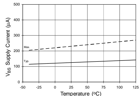
**Figure 17A. V<sub>Bs</sub> Supply Current vs. Temperature**
