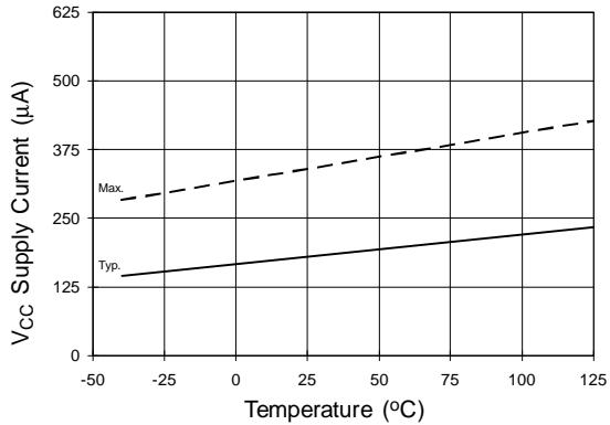
Figure 18A. V<sub>CC</sub> Supply Current vs. Temperature
