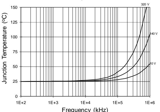
Figure 28. IRS2110/IRS2113 TJ vs. Frequency
