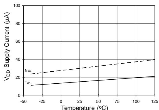
Figure 19A. V<sub>DD</sub> Supply Current vs. Temperature
