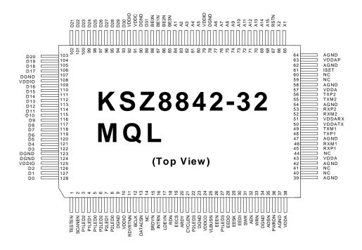
Figure 5. Standard - KSZ8842-32 MQL 128-Pin PQFP (Top View)
