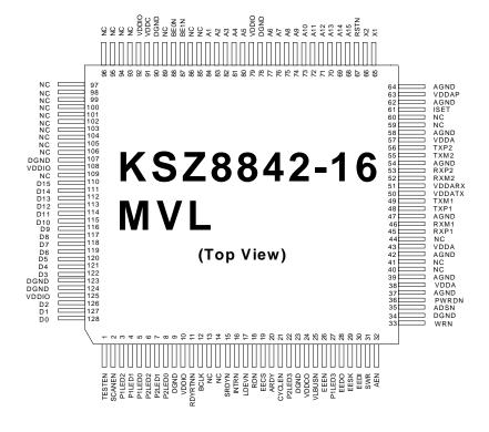
Figure 3. Option – KSZ8842-16 MVL 128-Pin LQFP (Top View)
