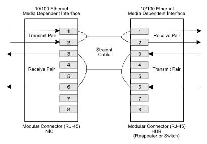
Figure 7. Typical Straight Cable Connection
