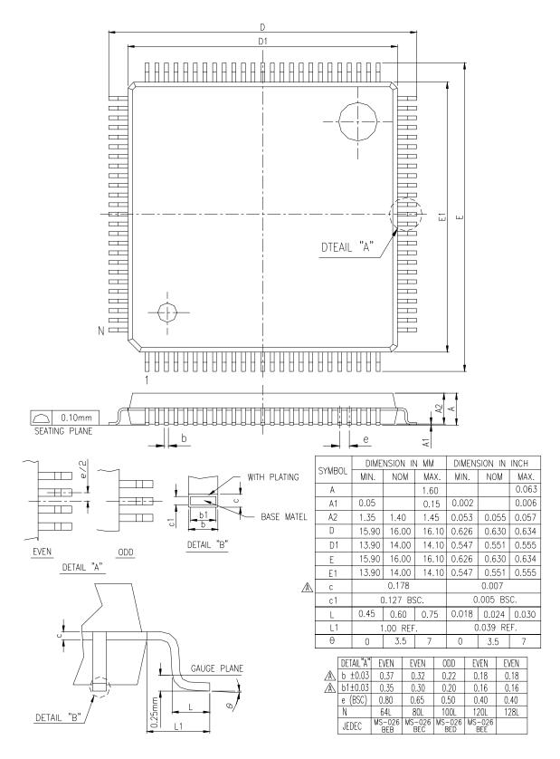
Figure 29. Optional 128-Pin LQFP Package
