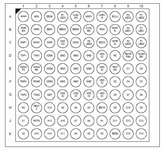
Figure 4. KSZ8842-16MBL 100-Ball LFBGA (Top View)
