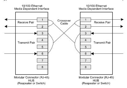
Figure 8. Typical Crossover Cable Connection
