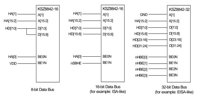
Figure 13. KSZ8842M 8-Bit, 16-Bit, and 32-Bit Data Bus Connections
