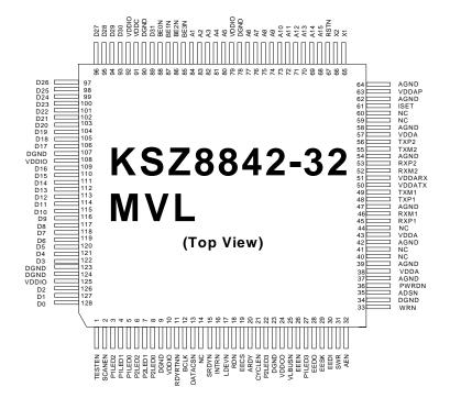
Figure 6. Option - KSZ8842-32 MVL 128-Pin LQFP (Top View)
