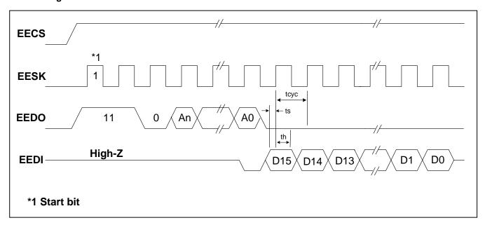
Figure 25. EEPROM Read Cycle Timing Diagram
