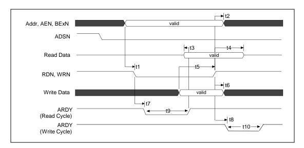
Figure 17. Asynchronous Cycle - ADSN = 0
