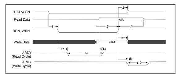
Figure 19. Asynchronous Cycle – Using DATACSN
