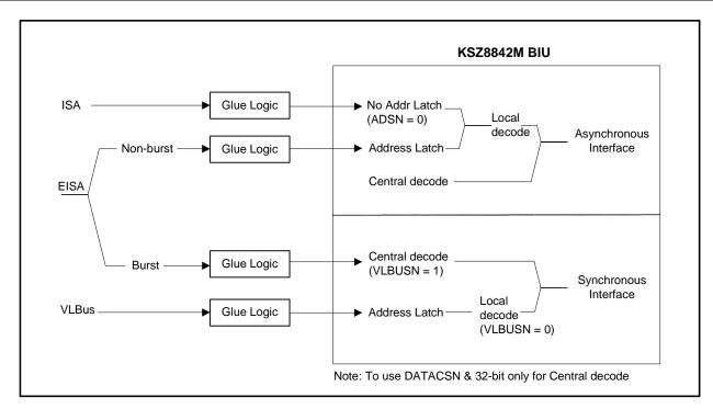
Figure 12. Mapping from ISA-like, EISA-like, and VLBus-like transactions to the KSZ8842M Bus
