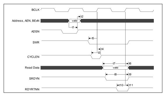
Figure 24. Synchronous Read Cycle – VLBUSN = 0
