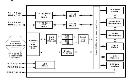
Figure 1. KSZ8842M Functional Diagram
