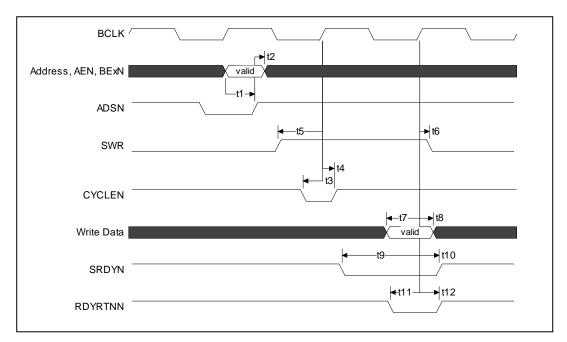
Figure 23. Synchronous Write Cycle – VLBUSN = 0
