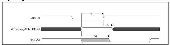
Figure 20. Address Latching Cycle for All Modes
