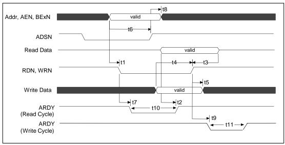
Figure 18. Asynchronous Cycle - Using ADSN
