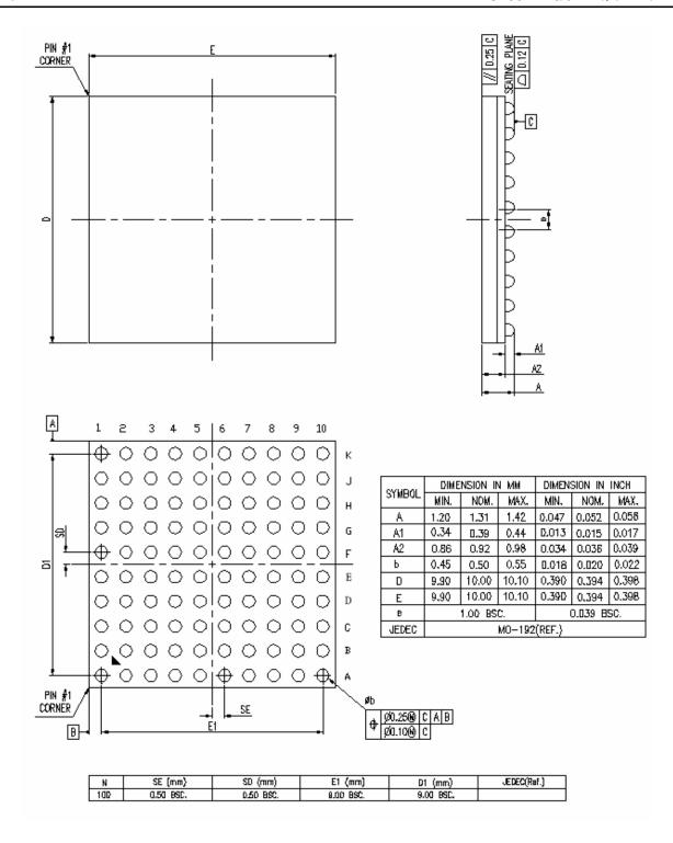
Figure 30. Optional 100-Ball LFBGA Package
