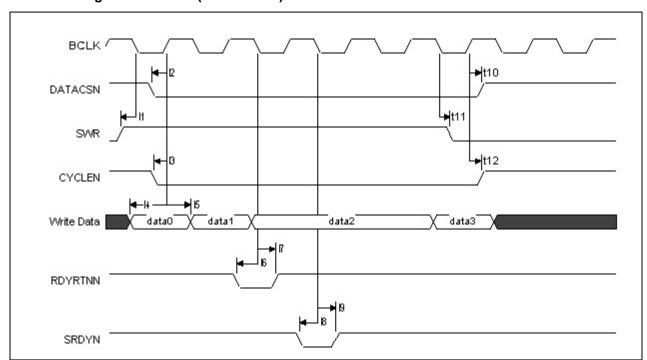
Figure 21. Synchronous Burst Write Cycles – VLBUSN = 1
