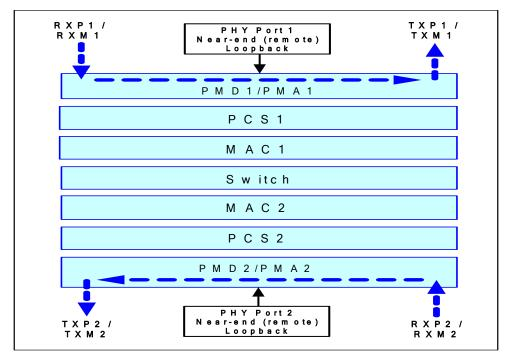
Figure 16. Port 1 and port 2 Near-End (Remote) Loopback Path
