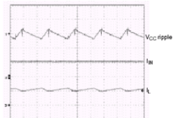
Figure 25. Boost Input Voltage and Current Ripple Waveforms
