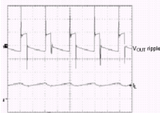
Figure 27. Typical Output Voltage Ripple
