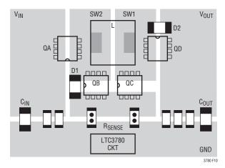
Figure 10. Switches Layout
