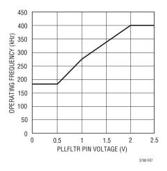
Figure 7. Frequency vs PLLFLTR Pin Voltage
