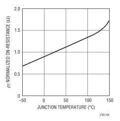
Figure 9. Normalized R<sub>DS(ON)</sub> vs Temperature
