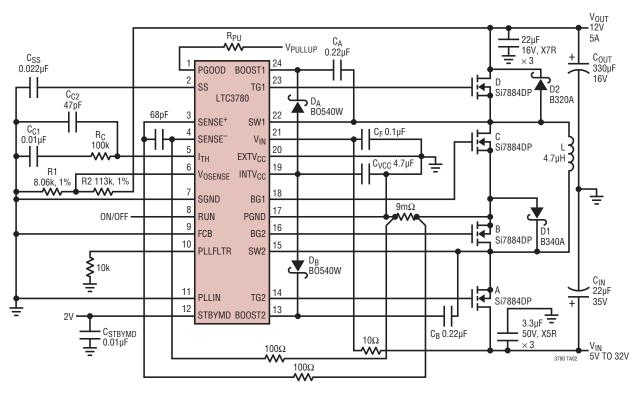
Figure 13. LTC3780 12V/5A, Buck-Boost Regulator
