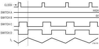
Figure 5. Boost Mode ( $V_{IN} < V_{OUT}$ )
