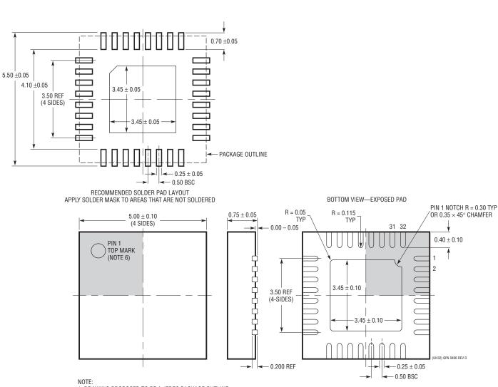
**UH Package** 32-Lead Plastic QFN (5mm  $\times$  5mm) (Reference LTC DWG # 05-08-1693 Rev D)
