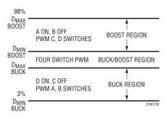
Figure 2. Operating Mode vs Duty Cycle
