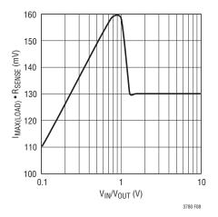
Figure 8. Load Current vs V<sub>IN</sub>/V<sub>OUT</sub>
