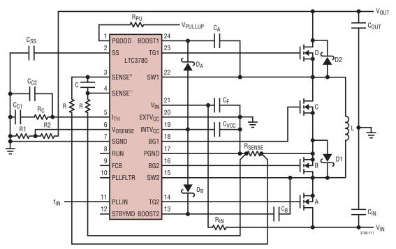
Figure 11. LTC3780 Layout Diagram
