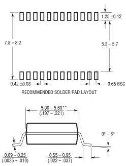
G Package 24-Lead Plastic SSOP (5.3mm) (Reference LTC DWG # 05-08-1640)
