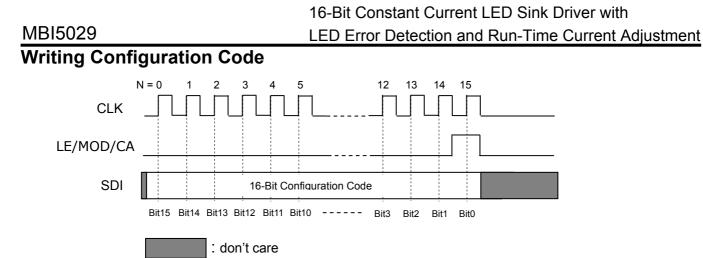
The second difference is that the active high signal LE/MOD/CA latches the serial data in the Shift Register to the Configuration Latch, instead of the Output Latch. The latched serial data is regarded as the Configuration Code. The code would be memorized until power off or the Configuration Latch is re-written. As shown above, the timing for writing the Configuration Code is the same as that in the Normal Mode for latching output channel data.
