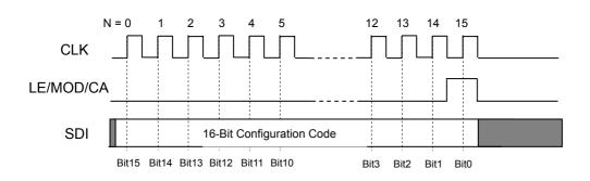
In the Special Mode, by sending the positive pulse of LE/MOD/CA, the content of the Shift Register with a Configuration Code will be written to the 16-bit Configuration Latch.
