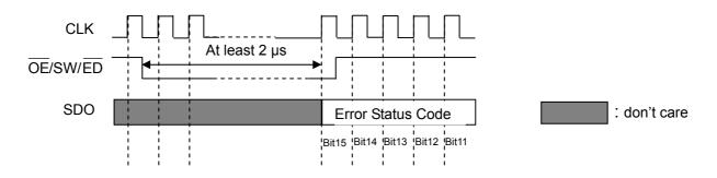
When MBI5029 is working in the Special Mode, the above signal sequence example can let a system controller read the Error Status codes via the pin SDO.
