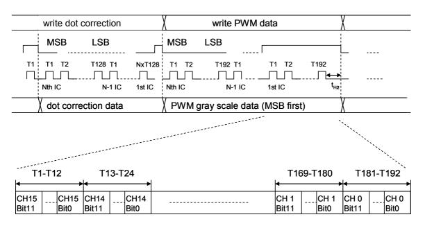
t<sub>H2</sub>: In the end of gray scale mode, DCLK -LE should be no less than 10ns.
