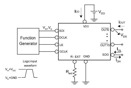
**Switching Characteristics (V<sub>DD</sub>=5.0V; Ta=25°C)**
