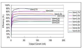
Fig. 14 Efficiency vs. Output Current
