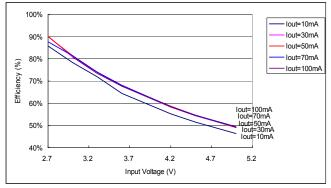
Fig. 13 Efficiency vs. Input Voltage
