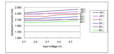
Fig. 9 Quiescent Current vs. Input Voltage
