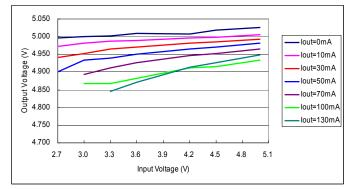
Fig. 7 Output Voltage vs. Input Voltage (C<sub>IN</sub>=C<sub>OUT</sub>=10uF, C<sub>FLY</sub>=1uF)
