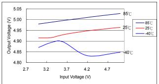
Fig. 10 Output Voltage vs. Input Voltage (I<sub>OUT</sub>=60mA)
