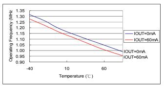
Fig. 12 Operating Frequency vs. Temperature (V<sub>IN</sub>=3.7V)
