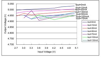
Fig. 8 Output Voltage vs. Input Voltage ( $C_{IN}=C_{OUT}=1uF$ ,  $C_{FLY}=0.1uF$ )
