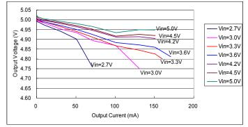
Fig. 5 Output Voltage vs. Output Current (C<sub>IN</sub>=C<sub>OUT</sub>=10uF, C<sub>FLY</sub>=1uF)
