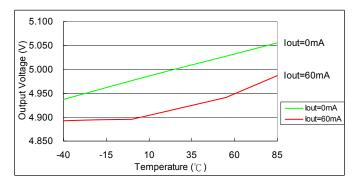
Fig. 11 Output Voltage vs. Temperature ( $V_{IN}$ =3.3V)
