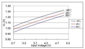
Fig. 16 V $_{\rm IL}$  vs. Input Voltage
