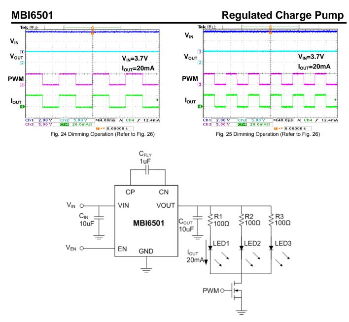
Fig. 26 Application circuit for backlight dimming
